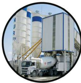
Concrete Batching & Mixing
